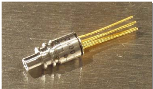
Photo showing ROSA with optional -30dB ORL receptacle (option: L3 or L4)
